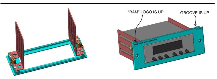
FACEPLATE ASSEMBLY PRIOR TO INSTALLING RADIO OR EQUIPMENT. WE SUGGEST CHECKING THAT THIS ASSEMBLY WILL FIT INTO THE TOUGH-BOX CONSOLE PRIOR TO ATTACHING THE RADIO OR EQUIPMENT JUST TO MAKE CERTAIN THE SIDE BRACKETS ARE CUT PROPERLY.
